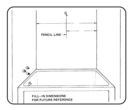
2. Accurately measure tub spout and handle(s) hole location on alcove side wall and transfer dimensions to one of the remaining flat panels. You may want to make a template (use shipping carton) to check hole layout before you cut holes into side panel. After you have double checked your measurements, using the proper size drill or hole saw, cut out holes for outlets.
